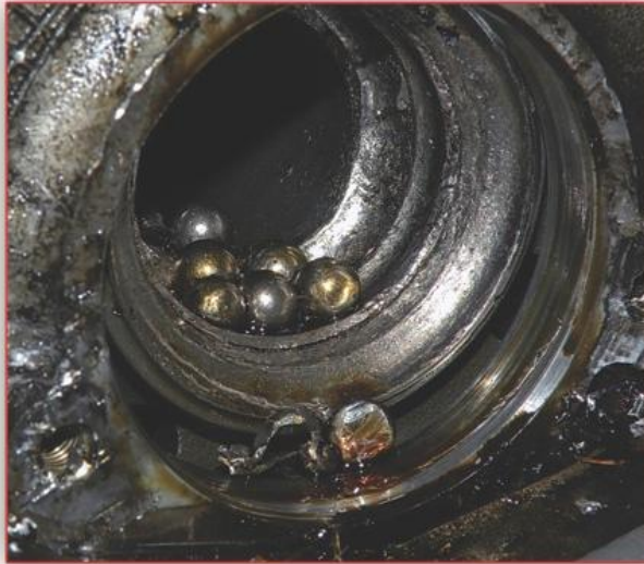
Catastrophic engine failure caused by IMS bearing failure
